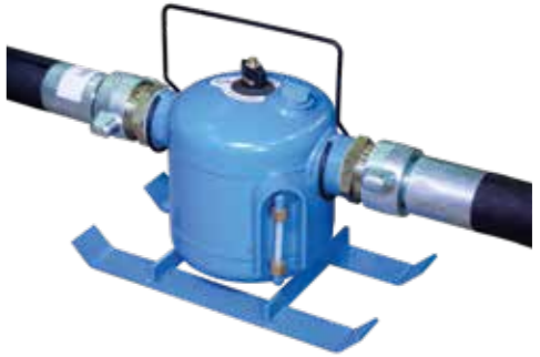
THE 7-L OIL LUBRICATOR is built in between the compressor and the machine to enable lubrication of the internal piston.
