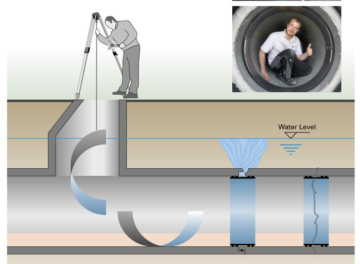
The QUICK-LOCK system is very well established for the rehabilitation of supply lines, especially in the field of drinking water. It doesn't matter whether it concerns vertical well piping or horizontal pressure piping, many partial damages can be repaired sustainable by QUICK-LOCK.
